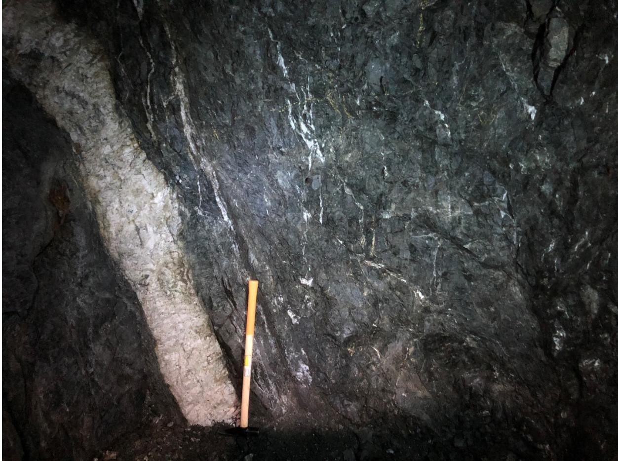
Figure 4.3 #4 vein drift showing a distinct 30 cm wide quartz-carbonate vein.
